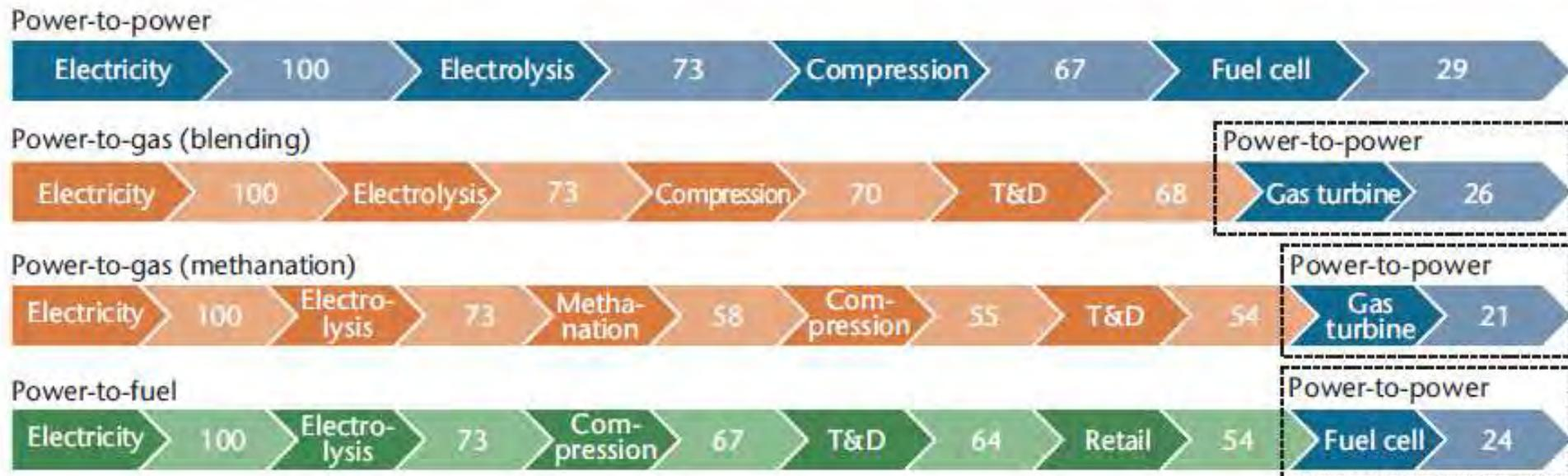
Note: The numbers denote useful energy; except for gas turbines, efficiencies are based on HHV; the conversion efficiency of gas turbines is based on LHV.
